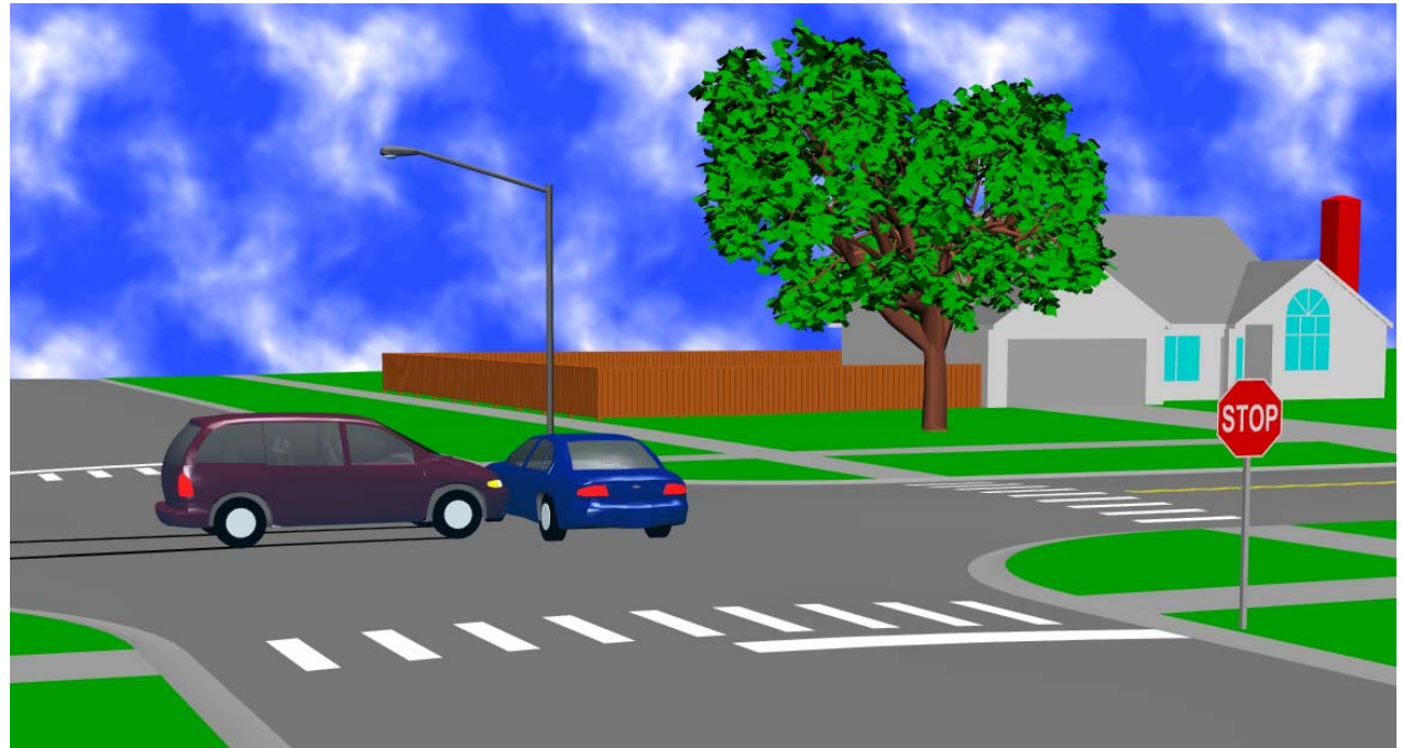
Still image from computer simulation of collision with environment constructed from Total Station data collection.
